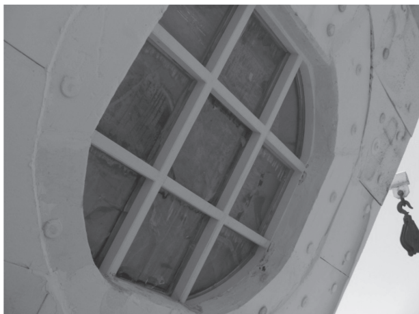
Fig. 4 SYN-PET500 reactor receiver window
