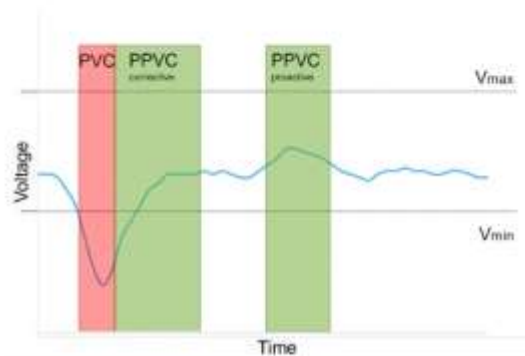
Fig. 1. Operation of PVC and PPVC
